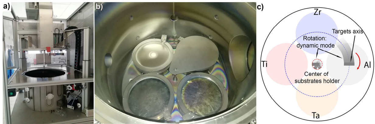
Figure 1. a) Magnetron sputtering system. b) Chamber, four targets configuration. c) Rotating substrates holder showing the two different substrates positions (center and targets axis).
