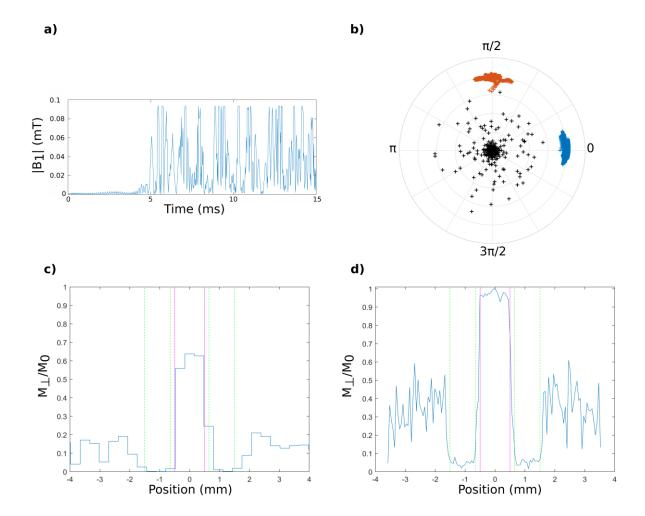
Figure 4. Numerical evaluation of the robustness of the OC pulse A ( $T2_{opt} = 30 \text{ ms}$ ) with respect to the variability of the sample T2-value. Final transverse magnetization states are presented in Bloch spheres when applying the OC pulse with and without motion for samples with T2-values of a) 5 ms and b) 90 ms. c) Simulated transverse magnetization amplitude and PNR variation with respect to sample T2-value.
