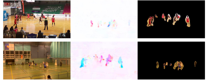
Figure 1: On the left column, images taken from a video. In the middle, optical flow computed from the left image and the previous frame. On the right, background/foreground segmentation.
