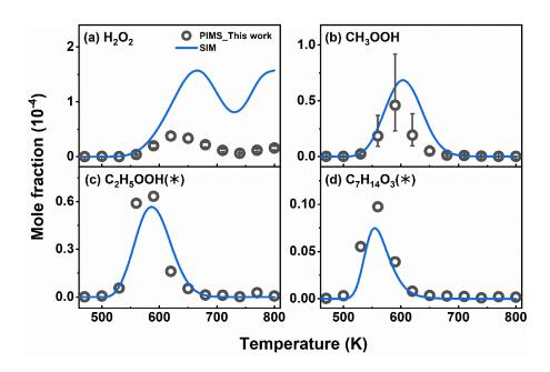
**Figure 4.** Experimental (symbols) and simulated (lines) profiles of  $H_2O_2$  (a), methyl hydroperoxide (b), ethyl hydroperoxide (c), and keto-hydroperoxides (d) in n-heptane low-temperature oxidation (P = 10 bar,  $\tau$  = 2 s,  $\phi$  = 1.0 and  $x_{fuel}^{inlet}$  = 0.001). Error bar for the experimental data in this work is given. The signal profiles (\*) of ethyl hydroperoxide and keto-hydroperoxides are presented.
