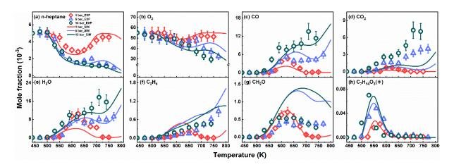
**Figure 5.** Experimental (symbols) and simulated (lines) profile of *n*-heptane, O<sub>2</sub>, CO, CO<sub>2</sub>, H<sub>2</sub>O, C<sub>2</sub>H<sub>4</sub>, CH<sub>2</sub>O, and keto-hydroperoxides in *n*-heptane low-temperature oxidation (P = 1, 5, and 10 bar,  $\tau = 2$  s,  $\phi = 1.0$  and  $x_{fuel}^{inlet} = 0.005$ ). Error bar for the experimental data in this work is given. Signal profile (\*) of keto-hydroperoxides is presented.
