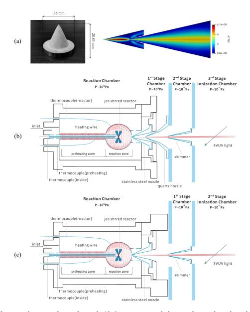
**Figure 1.** The stainless-steel nozzle with  $Al_2O_3$  coating and the mach number distribution map of the Ar after the sampling by the 50  $\mu$ m stainless steel nozzle and 250  $\mu$ m quartz nozzle (a), the schematic of the VP-JSR coupled to the SVUV-PIMS system at Combustion and Flame beamline (b), and at Atomic and Molecule Physics beamline (c) of Hefei Light Source.
