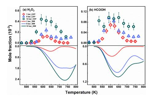
**Figure 6.** Experimental (symbols) and simulated (lines) profile of  $H_2O_2$  and formic acid in n-heptane low-temperature oxidation (P = 1, 5, and 10 bar,  $\tau$  = 2 s,  $\varphi$  = 1.0 and  $x_{fuel}^{inlet}$  = 0.005). Error bar for the experimental data in this work is given.
