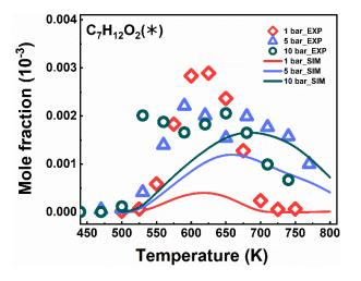
**Figure 7.** Experimental (symbols) and simulated (lines) profile of  $C_7H_{12}O_2$  in n-heptane low-temperature oxidation (P = 1, 5, and 10 bar,  $\tau$  = 2 s,  $\varphi$  = 1.0 and  $x_{fuel}^{inlet}$  = 0.005). Signal profile (\*) of  $C_7H_{12}O_2$  is presented.
