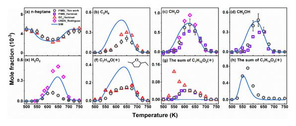
**Figure 2.** Data comparison of *n*-heptane low-temperature oxidation at 1 bar, in this work, with the measurement by Herbinet *et al.* [41] and Rodriguez *et al.* [27] (P = 1 bar,  $\tau$  = 2 s,  $\phi$  = 1.0 and  $x_{fuel}^{inlet}$  = 0.005). Error bar for the experimental data in this work is given. SVUV-PIMS data of C<sub>7</sub>H<sub>14</sub>O<sub>3</sub>, C<sub>7</sub>H<sub>12</sub>O<sub>2</sub>, and C<sub>7</sub>H<sub>14</sub>O<sub>3</sub> are signal profiles (\*).
