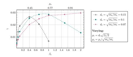
FIGURE 6. Numerical growth rates of the collisionless tearing mode as a function of  $\beta_e$  and  $\rho_s$ , for different values of  $d_e = \sqrt{m_e/m_i}$ . The box size is  $-\pi < x < \pi$ ,  $-0.47\pi < y < 0.47\pi$ , which leads to  $\Delta' = 0.59$ .
