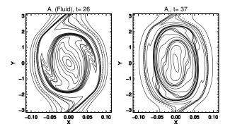
FIGURE 17. Contour plot of the Lagrangian invariant  $A_-$ . Left panel:  $\beta_e = 0$ , right panel:  $\beta_e = 1.5$ . The parameters are  $d_e = 0.06$ ,  $\rho_s = 0.519$ . The dashed lines are the separatrices. The contour plots refer to the normalized time  $\gamma t = 5.18$
