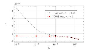
FIGURE 8. Comparison between the linear growth rate obtained in the cold-ion regime and the hot-ion regime. The box size is  $-\pi < x < \pi$ ,  $-0.47\pi < y < 0.47\pi$ , which leads to  $\Delta' = 0.59$ .
