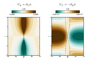
FIGURE 12. Contour plot of the perpendicular velocity component for  $\beta_e = 0$ . On the left:  $U_y$ . On the right:  $U_x$ . The parameters are the same as those on Fig. 11. The magnetic island edges are shown by the dotted lines. Not the entire domain is shown.
