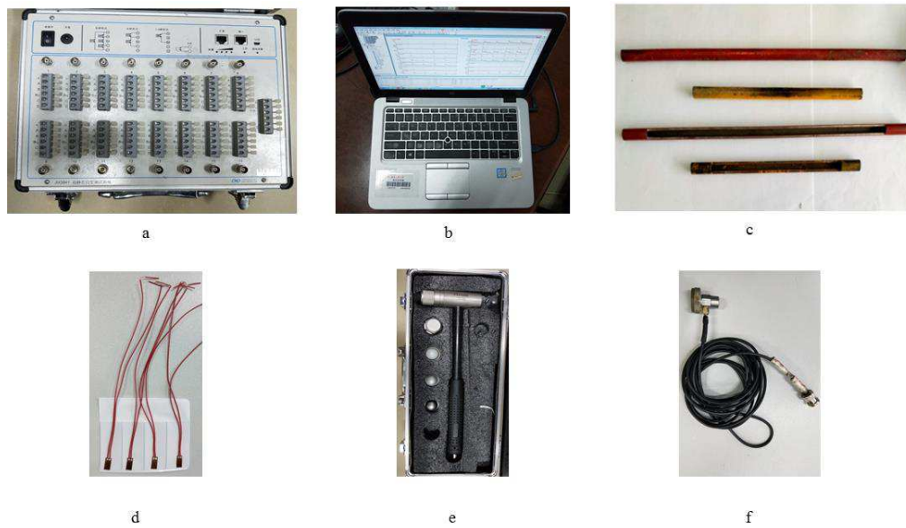
Fig. 8. Experimental devices. (a) Acquisition instrument, (b) Laptop, (c) Intact and damaged rods, (d) Strain gage, (e) Impact hammer, (f) Accelerometers.
