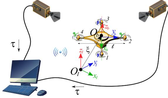
Figure 3.1: Quadrotor vehicle and vision-based tracking system (scheme conceived from figures available at [freepik.com](http://freepik.com))
