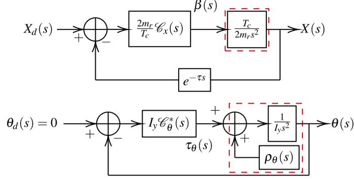
Figure 5.1: Block diagram representation of the quadrotor with tilting-rotors closed-loop system
