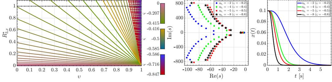
Figure 4.2: (left) Behavior of  $R_{3,x}^*(\varsigma; v)$  within the interval  $0 < v < 1$ . Numerical evidence of the dominance of the root  $s_{0_x}$  within the intervals in (4.53)-(4.55) with  $\tau = 0.1$  [s]: (Center) Spectral distribution of the roots. (Right) Time-domain solution.
