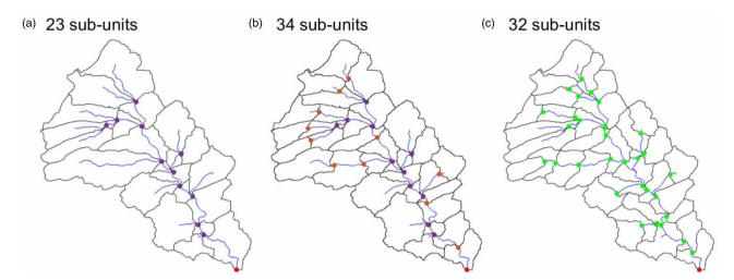
Figure 7 | (a) Partition at confluences (magenta dots), (b) additional partition with respect to a reach length of 2 km (orange dots) and (c) unguided area-balanced partition (green dots).
