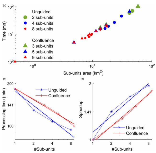
**Figure 11** | DDM computing times with respect to sub-units. (a) Computation time per basin for the unguided area-balanced partition (triangles) and the confluence partition (filled circles), (b) processing time, and (c) speed-up for different partitions.
