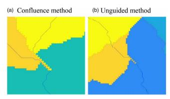
Figure 4 | Isolated cells near to outlets. (left) Partition method at confluences and (right) unguided area-balanced partition method.
