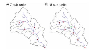
Figure 3 | Guided partitioning. (a) User-defined points (red dots) and (b) partition of the largest watershed into two sub-watersheds of a similar area (green dot).
