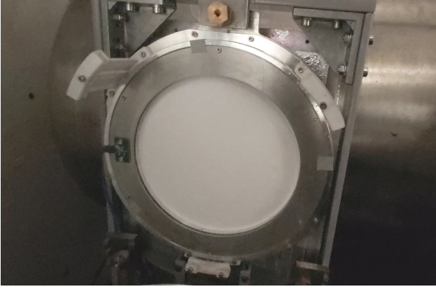
Fig. 23. M-HWP C device mounted in front of the NIKA2 instrument.
