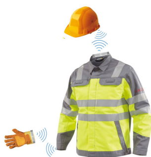
FIGURE 21. Example of a potential T2T system. The illustrated idea is to detect a potential misplacement (or even absence) of the safety equipment, and thus, the user is warned.
