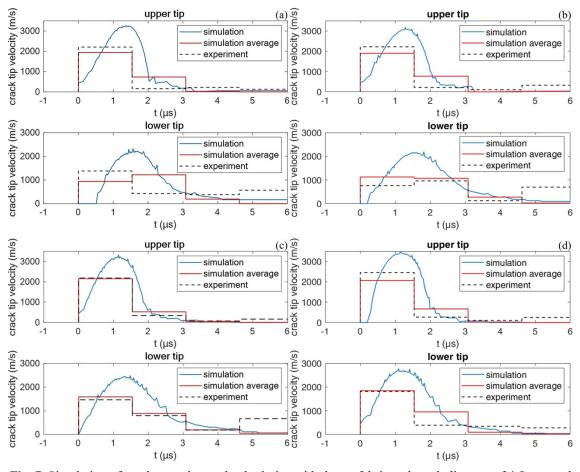
**Fig. 7.** Simulation of crack growth speed at both tips with the prefabricated crack distance of 4.5 mm and the prefabricated crack angle of (a) 0, (b) 26.6, (c) 45 and (d) 63.4° during flame thermal shock.
