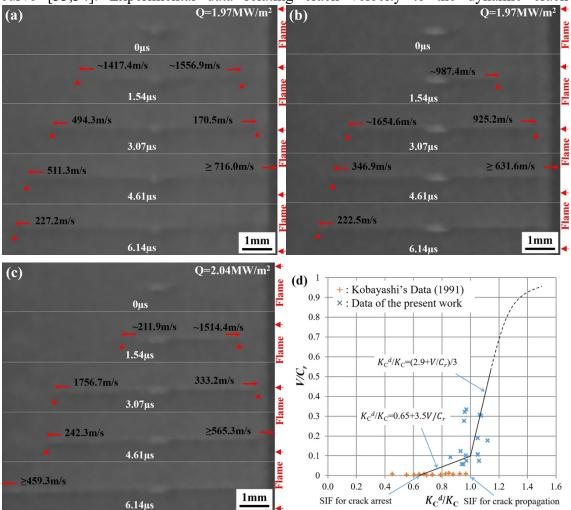
**Fig. 4.** Measured crack growth speeds of (a) specimen 1, (b) specimen 2, (c) specimen 3 for identification, with the speed error of 50.7m/s, and (d) Estimation of the  $K_{\rm C}^d - V$  relationship.
