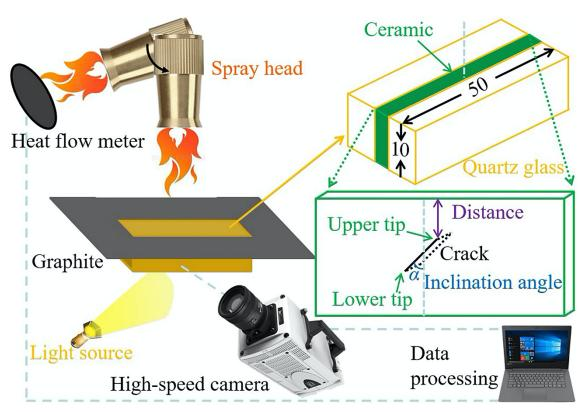
Fig. 1. Schematic diagram of processing sample and observation device for flame thermal shock.
