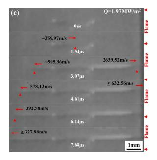
**Fig. 8.** Thermal shock crack propagation process during flame thermal shock when the upper tip distance of prefabricated crack is (a) 3, (b) 4, and (c) 6 mm, with the speed error of 50.7m/s.
