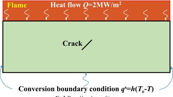
Fig. 2. Thermal boundary conditions.
