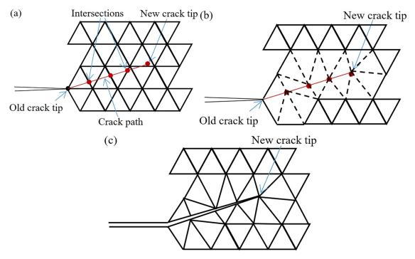
Fig. 3. Re-meshing procedure. (a) find the crack path and the intersection points, (b) move the nearest nodes to the intersection points, (c) doubling the intersection nodes to form the new mesh near the moving crack tip.
