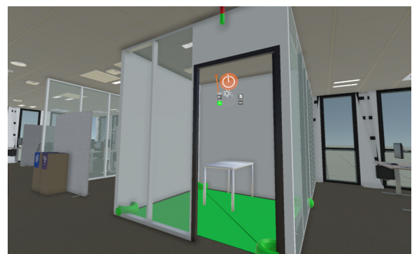
Figure 3: An example of augmentation for controlling a connected light. This augmentation is part of an augmentation layer. The green polygon corresponds to the area where this augmentation will be visible from the user.
