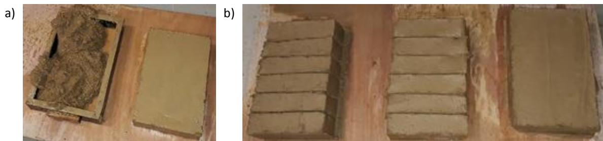
Figure 2. Construction of specimens: a) casting earth into mould, b) specimens after wire cutting, the third slab is cut after drying
