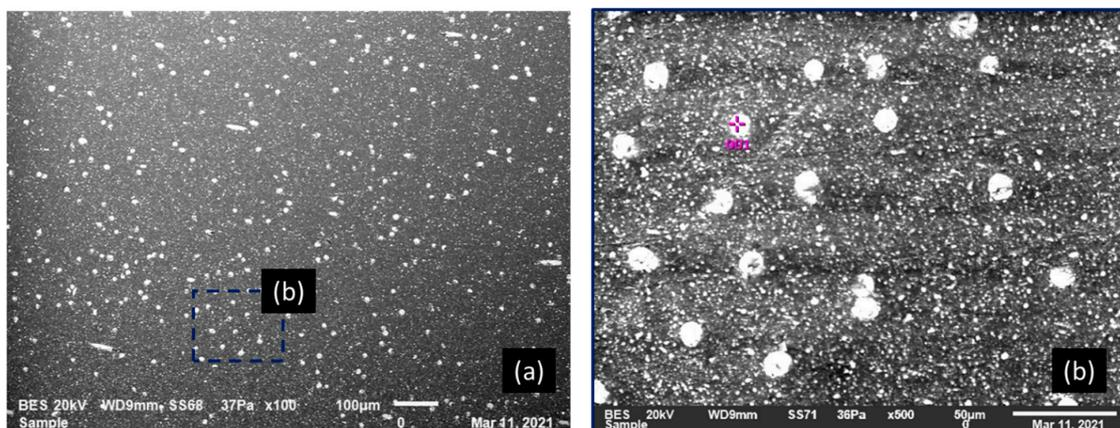
**Figure 9.** SEM micrographs of the transverse surface of a fractured tensile test sample with 5% GF/PBT composite, 20 kV, 9 mm working distance, 36 Pa: (a) BES macro-image; (b) fiber distribution on PBT matrix.
