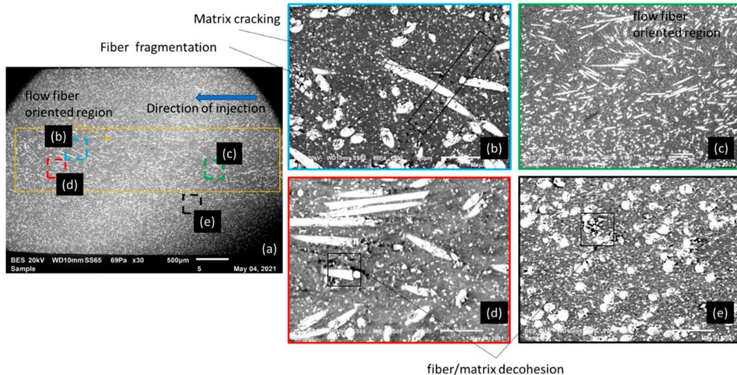
**Figure 8.** SEM micrographs of the transverse surface of a fractured tensile sample with 30% GF/PBT composite, 20 kV, 10 mm working distance, 69 Pa: (a) BES macro-image with flow fiber-oriented region; (b–d) zoom of different regions in the zone (a); (e) homogeneous zone.
