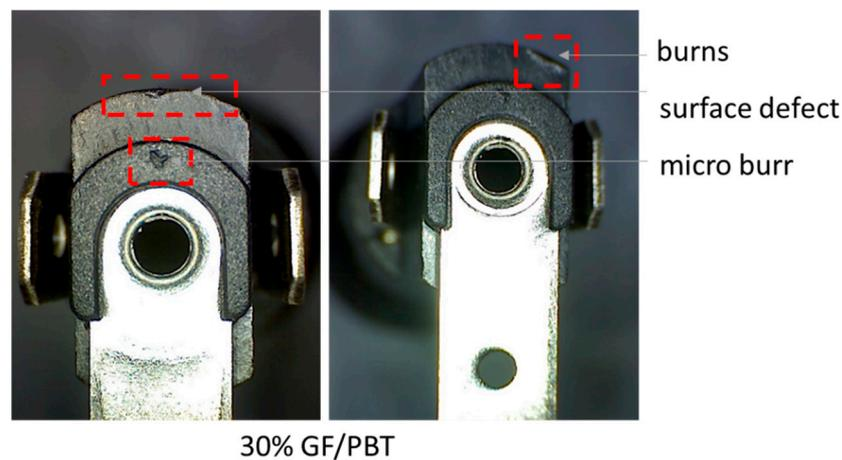
**Figure 15.** Optical image of micro-faults on 30% GF/PBT composite.
