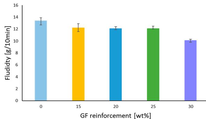
Figure 14. Fluidity vs. GF reinforcement rate.
