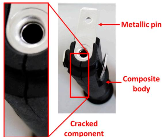
**Figure 1.** Crack in the considered electrical component.
