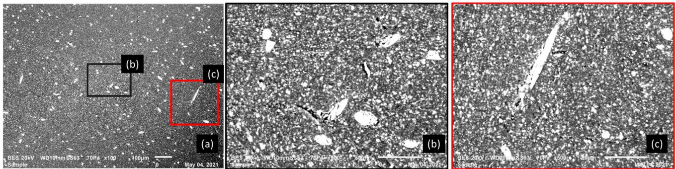
**Figure 10.** SEM micrographs of the transverse surface of a fractured tensile test sample with 5% GF/PBT composite, 20 kV, 10 mm working distance, 70 Pa: (a) BES macro-image; (b,c) zoom of different regions in the zone (a).
