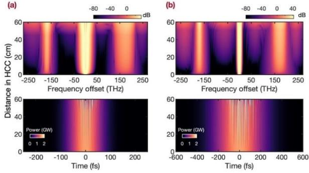
Fig.7 Spectral and temporal evolutions along the HCC, for case I.b (a) and II.a (b) at a pressure of 1.2 bar.
