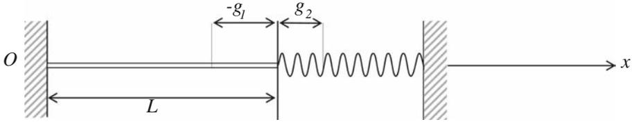
FIG. 1. The rod–spring system with unilateral constraints
