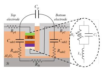
Fig. 2: Integrated STD device and related equivalent electrical elements.
