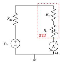
Fig. 4: DC characterization set-up for STD device.
