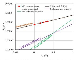
Fig. 5: Measured  $I_{dc}(V_{dc})$  STD characteristics (red) and 3-rd order polynomial fit (black).
