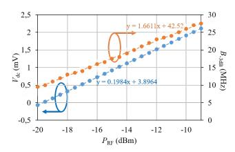
Fig. 11: Measured output DC voltage,  $V_{dc}$ , and -3dB bandwidth,  $B_{-3dB}$ , of the STD as a function on the input RF power in dBm,  $P_{RF}(dBm)$ . Linear interpolations are represented with dashed lines.
