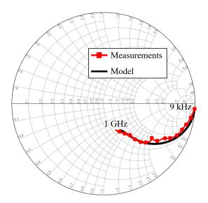
Fig. 7: Measured and simulated  $S_{11\text{open}}$  reflection coefficient for the reference open circuit in the frequency range [9 kHz - 1 GHz].
