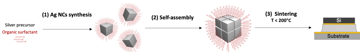
Scheme 1. Scheme Showing the Low-Temperature (LT) Fabrication of Silver Joint Investigated in This Study Following Three Steps: (1) Colloidal Synthesis of Nanocubes (2) Self-Assembly into Close-Packed Supercrystals by Drop Casting (3) Thermal Annealing Treatment to Induce the Sintering into Dense Joints.
