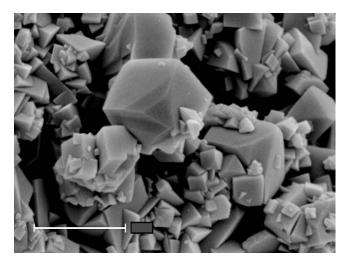
Fig. 1. Scanning electron microscope (SEM) images of synthetic Pb-jarosite. Scale bar equals 1  $\mu$ m. The image was taken at 35,000× magnification, spot size 3.0, and 5 kV accelerating voltage.
