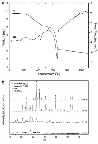
Fig. 2. (a) TG–DTA profiles of synthetic Pb-jarosite (b) Powder XRD patterns for the thermal decomposition of synthetic Pb-jarosite under argon at 490, 585, 730, and 1080 °C (Cu K $\alpha$  radiation,  $\lambda = 1.54056$  Å).
