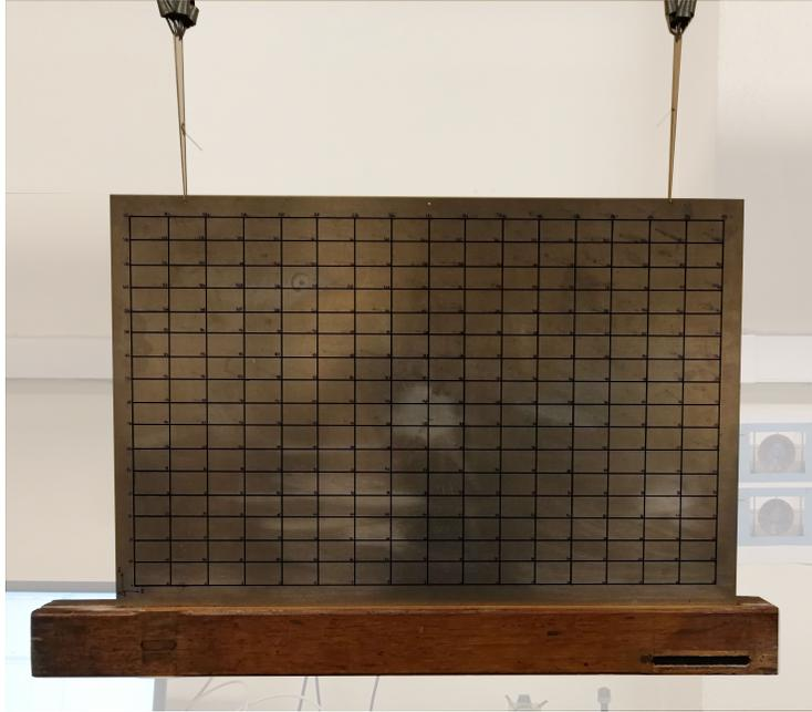
Figure 17: Structure under test – Definition of the grid of excitation points
