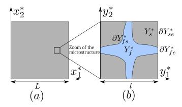
Figure 1: Schematic representation of a porous medium with periodic microstructure. a) Macroscopic scale. b) Elementary reference cell.
