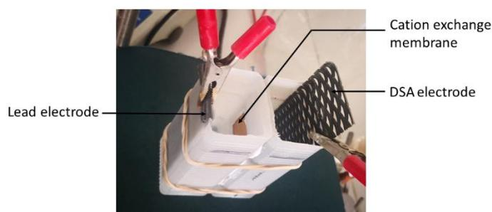
**Fig. 1.** Electrochemical cell with separated compartments
