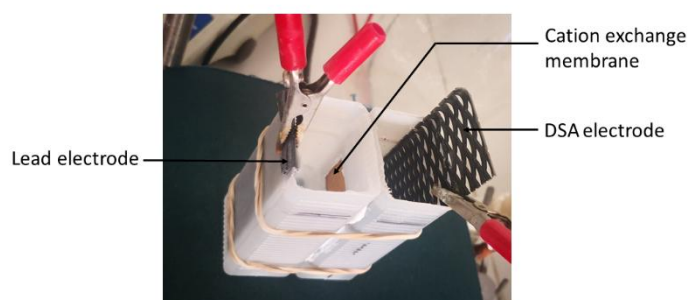
Fig. 1. Electrochemical cell with separated compartments
