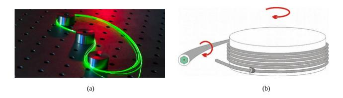
Figure 1. Examples of special coiling methods used for improving the mode-mixing and correspondingly the pump absorption in double clad fibers: (a) kidney shape coil and (b) simultaneous coiling and twisting of the active fiber.
