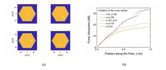
Figure 4. (a) Cross sections of the hexagonal fiber with a non-concentric core at different positions. (b) Evolution of the pump absorption along the propagation with a coiled and twisted double clad fiber for different position of the center of the core. The offset core leads to higher pump absorption.
