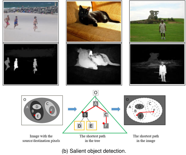
Fig. 1: Image processing with the max-tree. (a) Background extraction for document image analysis with a morphological black top-hat. The min-tree is pruned by removing connected small peak components ( < 4 pixels that do not touch the border). The residue (filtered components) forms the clean text and the background is removed. (b) Salient object detection for scene analysis [1]. A morphological tree is used to compute the Dahu distance from image borders. This distance that mixes geodesic distance and gray-level distances can be computed using a tree similar to the max-tree (the tree of shapes).
