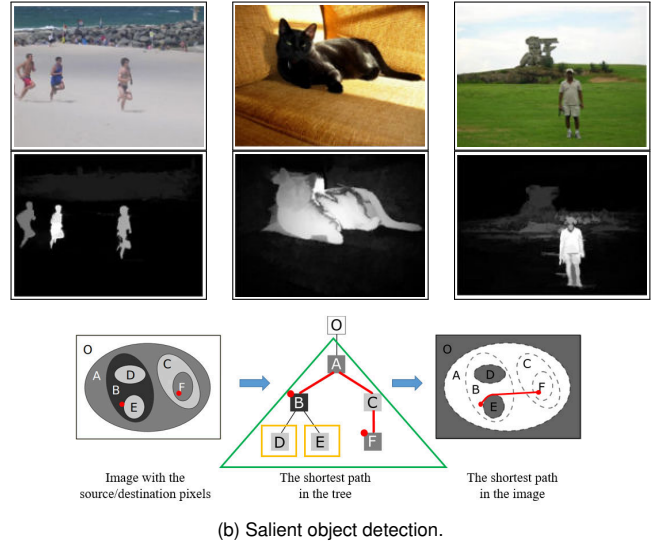
Fig. 1: Image processing with the max-tree. (a) Background extraction for document image analysis with a morphological black top-hat. The min-tree is pruned by removing connected small peak components ( < 4 pixels that do not touch the border). The residue (filtered components) forms the clean text and the background is removed. (b) Saliest object detection for scene analysis [1]. A morphological tree is used to compute the Dahu distance from image borders. This distance that mixes geodesic distance and gray-level distances can be computed using a tree similar to the max-tree (the tree of shapes).
