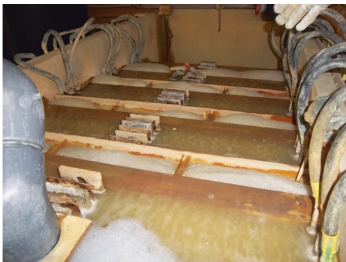
Fig. 3.3 Electrocoagulation unit at the industrial scale (Copyright: G. Crini, Besançon, France)
