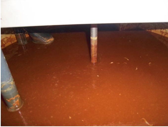
Fig. 3.2 An iron coprecipitation unit at an industrial scale (Copyright: G. Crini, Besançon, France)
