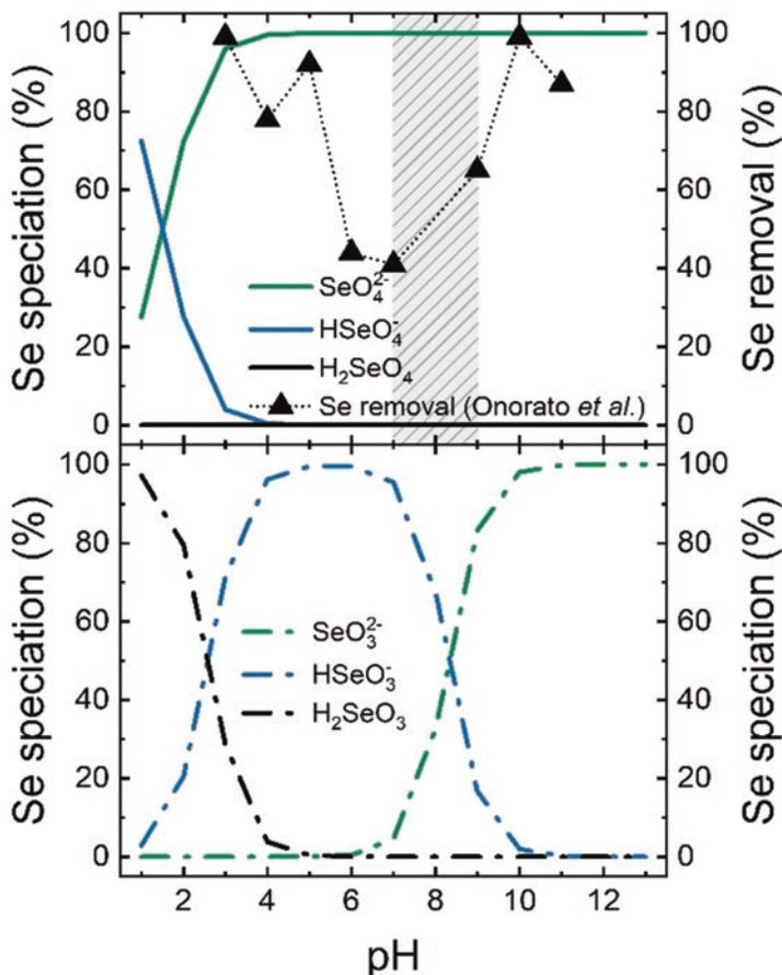
**Fig. 3.10** Speciation of selenium VI (top) and IV (bottom) over pH 1 to 13 and removal of selenium VI, adapted from Onorato et al. (2017); electric potential 12 V; feed salinity 5.3 g/L; membranes Neosepta CMX-SB & AMX-SB, Tokuyama Soda Ltd., Japan; the highlighted pH range shows the real pH of sample water used which was then modified by adding HCl and NaOH)
