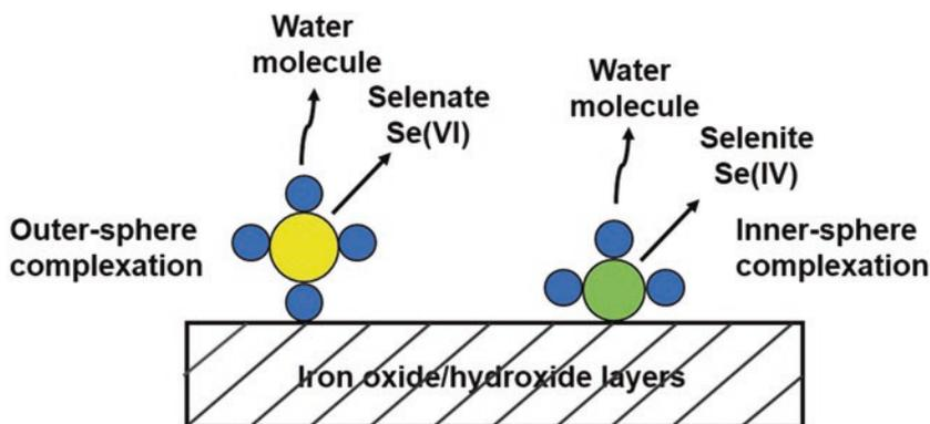
**Fig. 3.5** Selenate and selenite adsorption onto iron oxide and hydroxides. (Adapted from Hayes 1987)
