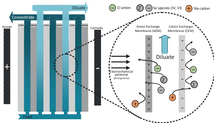
**Fig. 3.9** Principle of an electrodialysis process. (Source: Mehran Aliaskari, Eggenstein-Leopoldshafen, Germany)
