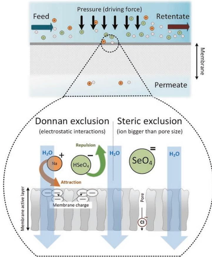
**Fig. 3.6** Mechanisms of ion rejection in nanofiltration/reverse osmosis. (Source: Youssef-Amine Boussouga, Eggenstein-Leopoldshafen, Germany)
