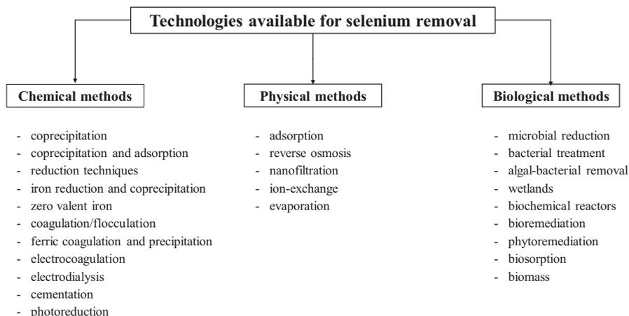
**Fig. 3.1** Classification of the technologies for selenium removal
