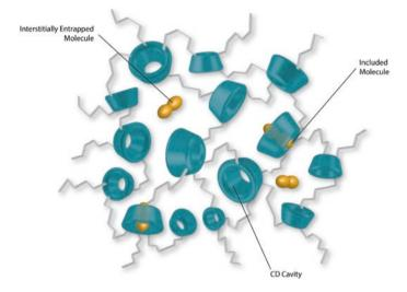
**Fig. 4.5** Illustration of the role of cyclodextrin cavities and the 3D polymer network during the complexation of a pollutant by a cyclodextrin polymer
