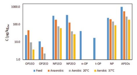
**Fig. 4.10** Concentration pattern of alkylphenol ethoxylates and related metabolites in the fed sludge and in the digested sludge after the anaerobic and aerobic digestion for the two operating conditions: anaerobic mesophilic-aerobic at T = 20 °C (AA20) and anaerobic mesophilic-aerobic at T = 37 °C (AA37)
