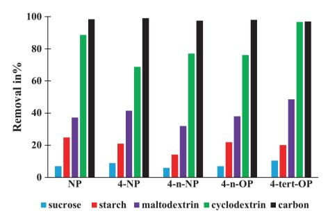
**Fig. 4.6** Comparison of different materials for the removal (in %) of several alkylphenols (NP: nonylphenol, mixture, CAS number 25154-52-3; 4-NP: 4-nonylphenol, mixture, CAS number 84852-15-3; 4-*n*-NP: linear *para*-nonylphenol, CAS number 104-40-5; 4-*n*-OP: linear para-octylphenol, CAS number 1806-26-4; 4-*tert*-OP: *para*-octylphenol, CAS number 140-66-9; adsorbent dose 2 g/L; initial concentration 100 μg/L; contact time 4 h; agitation 250 rpm; T 25 °C; pH 6; n = 2)
