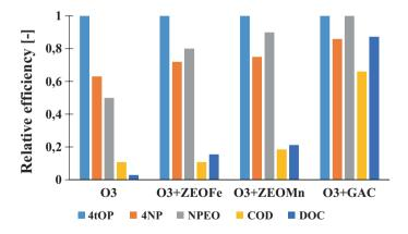
**Fig. 4.12** Efficiencies of several applied advanced oxidation processes (*O3* ozone, *ZEO* zeolite, *ZEOFe* Fe-modified zeolite, *ZEOMn* Mn\_modified zeolite, *GAC* granular activated carbon, *4tOP* 4-*tert*-octylphenol, *4NP* 4-nonylphenol, *NPEO* nonyphenol polyethoxylates, *COD* chemical oxygen demand, *DOC* dissolved organic carbon)
