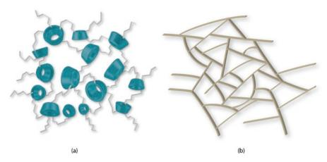
Fig. 4.4 Comparison of the structure of (a) a cross-linked epichlorohydrin cyclodextrin polymer and (b) a cross-linked epichlorohydrin dextran resin (Sephadex®)
