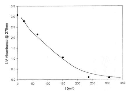
Fig. 4.15 Photodegradation of a 1000 ppm aqueous solution of nonylphenol ethoxylate by  ${\rm TiO_2}$  at pH 7
