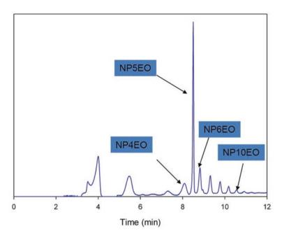
**Fig. 4.16** High performance liquid chromatogram of a nonylphenol pentaethoxylate (NP5EO) solution with UV-irradiated PEG-templated SiO<sub>2</sub>-TiO<sub>2</sub> (time = 90 min, *NP4EO* nonylphenol tetraethoxylate, *NP6EO* nonylphenol hexaethoxylate, *NP10EO* nonylphenol decaethoxylate)
