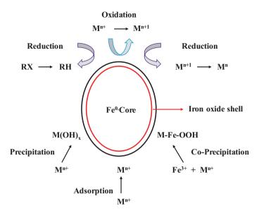
Fig. 4.17 Schematic illustration of zero-valent iron surface reactions
