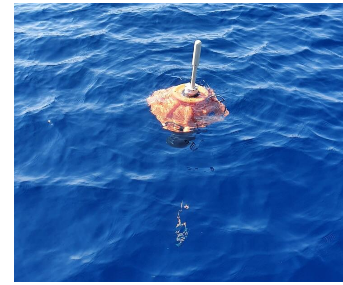
The MERMAID lander with its anchoring system during a test in the Mediterranean Sea.
