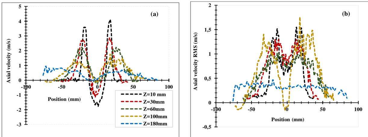
Figure 5. (a) Profiles of axial velocity of non reacting flow for 5 heights, Sn=1.4 and  $\phi=0.8$ . (b) Profiles of axial velocity RMS of non reacting flow.
