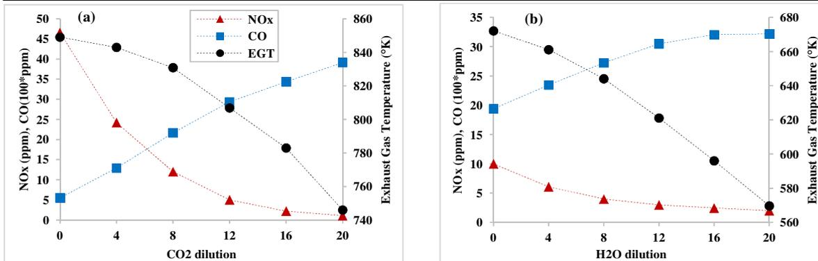
Figure 2. NOx, CO and EGT: (a): as function of CO<sub>2</sub>, at 25%O<sub>2</sub>,  $\phi=0.8$  and Sn=1.4. (b): as a function of H<sub>2</sub>O dilution at 21%O<sub>2</sub>,  $\phi=0.8$  and Sn=1.4
