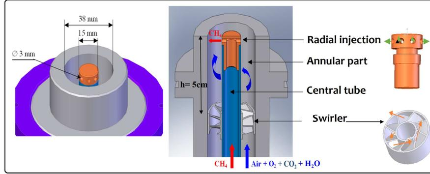
Figure 1. Coaxial swirl burner
