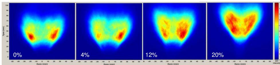
Figure 3. OH\* intensity distributions of H<sub>2</sub>O diluted CH<sub>4</sub>/air swirling flames at  $\phi=0.8$  and Sn=0.8
