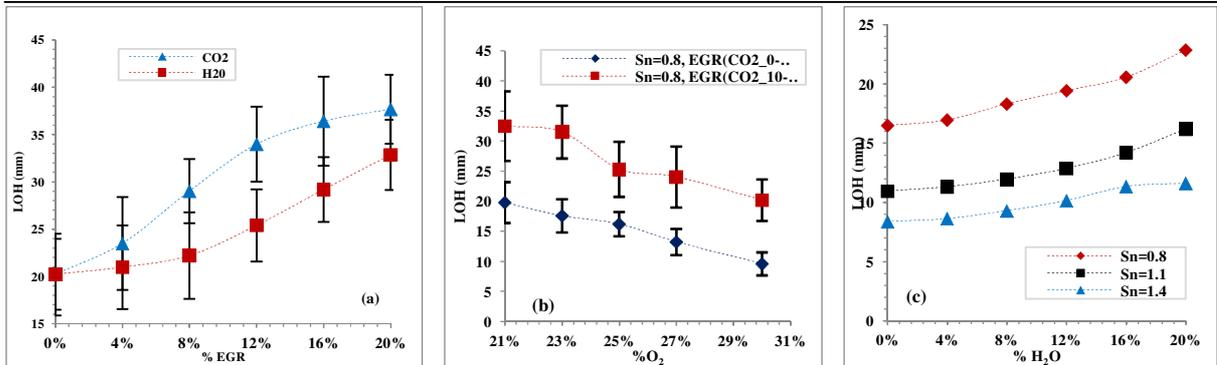
Figure 4. (a). Lift-off height with CO<sub>2</sub> and H<sub>2</sub>O dilutions for  $\phi=0.8$ , Sn=0.8 and 21%O<sub>2</sub>; (b): Lift-off height with O<sub>2</sub> enrichment with and without EGR; (c): lift-off heights with swirl/water vapor dilution for  $\phi=0.8$  and 25%O<sub>2</sub>.
