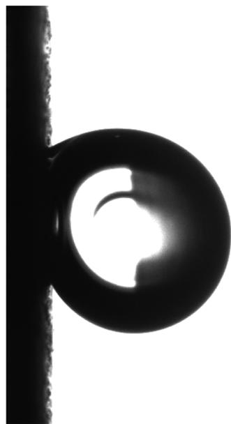
**Figure 7.** Picture of a water droplet on a surface inclined to 90° obtained with EDOP-*br*-C<sub>18</sub> and with a deposition charge of 400 mC cm<sup>-2</sup>. The droplet has a volume of 6 μL.
