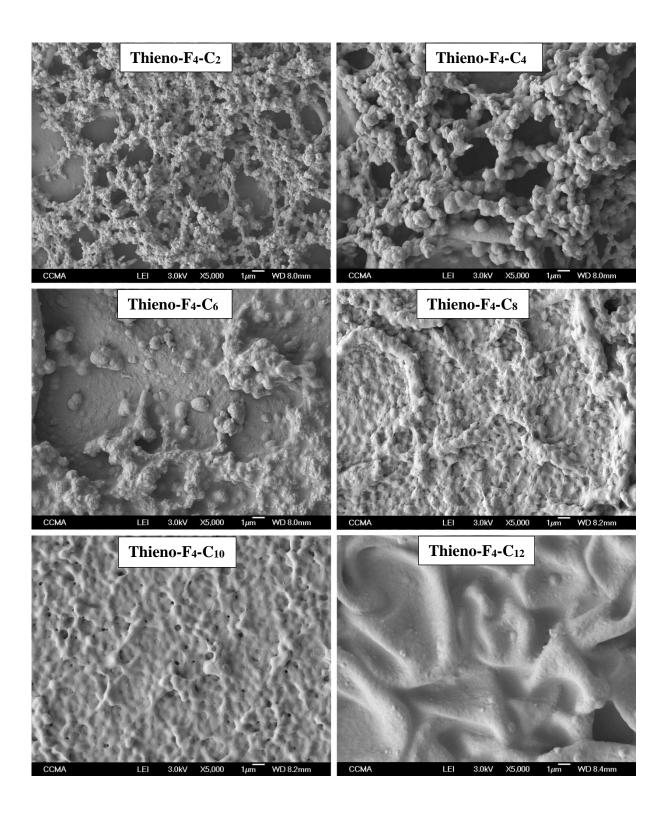
**Figure 3.** SEM images of polymer surfaces obtained from Thieno-F<sub>4</sub>-C<sub>2</sub>, Thieno-F<sub>4</sub>-C<sub>4</sub>, Thieno-F<sub>4</sub>-C<sub>6</sub>, Thieno-F<sub>4</sub>-C<sub>8</sub>, Thieno-F<sub>4</sub>-C<sub>10</sub> and Thieno-F<sub>4</sub>-C<sub>12</sub> with the solvent CH<sub>2</sub>Cl<sub>2</sub> and by cyclic voltammetry (3 scans).
