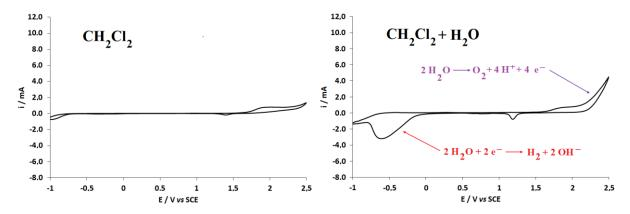
**Figure 1.** Cyclic voltammograms (1 scan) of the solvents  $CH_2Cl_2$  (left column) and  $CH_2Cl_2 + H_2O$  (right column) with  $Bu_4NClO_4$  as electrolyte. Scan rate: 20 mV s<sup>-1</sup>.
