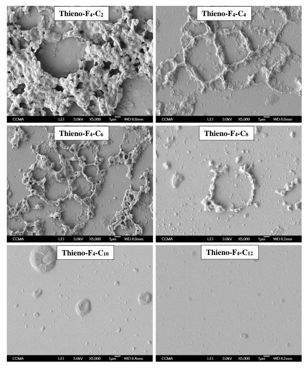
**Figure 5.** SEM images of polymer surfaces obtained from Thieno-F<sub>4</sub>-C<sub>2</sub>, Thieno-F<sub>4</sub>-C<sub>4</sub>, Thieno-F<sub>4</sub>-C<sub>6</sub>, Thieno-F<sub>4</sub>-C<sub>8</sub>, Thieno-F<sub>4</sub>-C<sub>10</sub> and Thieno-F<sub>4</sub>-C<sub>12</sub> with the solvent  $CH_2Cl_2 + H_2O$  and by cyclic voltammetry (3 scans).
