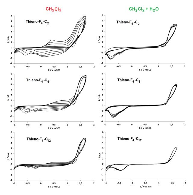
**Figure 2.** Electropolymerization curves of some of the monomers (0.01 M) in CH<sub>2</sub>Cl<sub>2</sub> or CH<sub>2</sub>Cl<sub>2</sub> + H<sub>2</sub>O / Bu<sub>4</sub>NClO<sub>4</sub> (0.1 M); 5 scans at a scan rate of 20 mV s<sup>-1</sup>.
