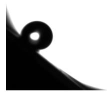
**Figure 4.** Picture of a water droplet on poly(**Thieno-F4-C**<sub>6</sub>) (5 scans) coated-substrate with an inclination of 45°.
