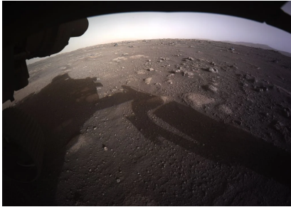
Fig. 1. First high-resolution color image sent by Hazard Cameras (Hazcams) of NASA’s Perseverance Mars vehicle after its landing on February 18, 2021. Distortion effects are in particular visible through the curved horizon line. Photo: NASA / JPL-Caltech.
