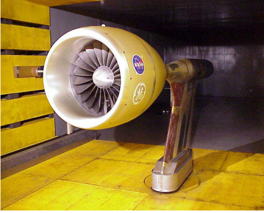
Fig. 1: NASA SDT model installed in the NASA Glenn Wind Tunnel
