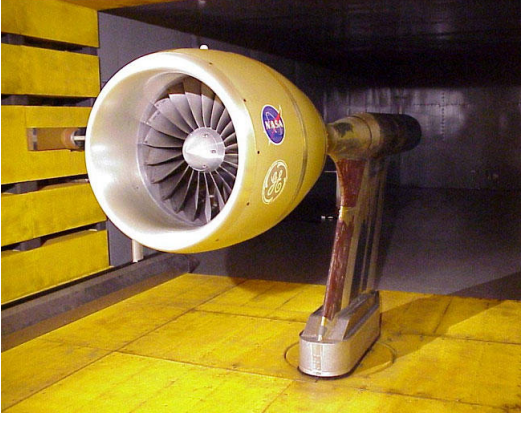
Fig. 1: NASA SGT model installed in the NASA Glenn Wind Tunnel
