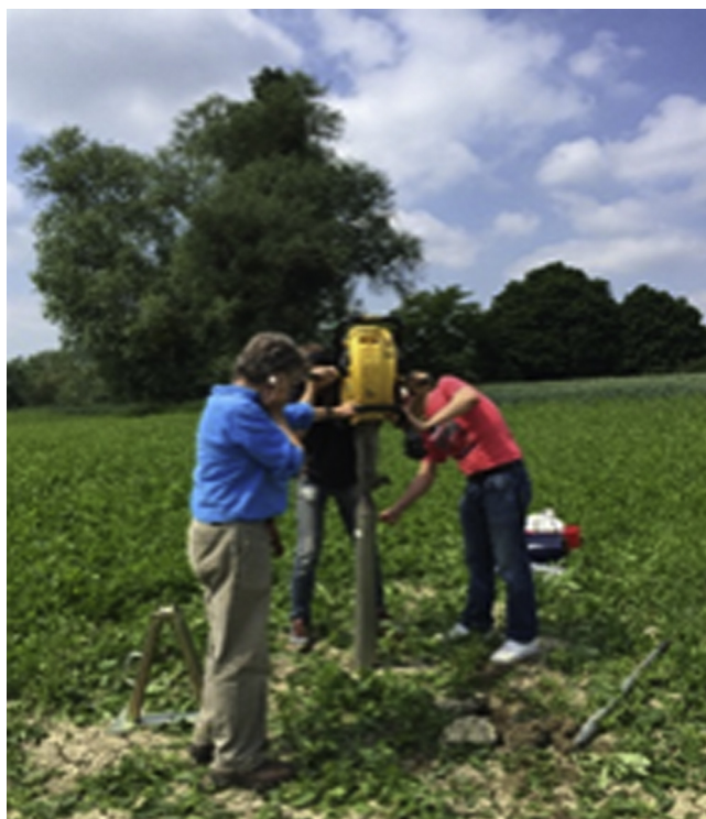
PHOTO 5.2.2 Floodplain sediment sampling by portable corer at Bouafles on May 23, 2018 (see location on Fig. 5.2.1). The Seine River channel is at 30–40 m. Credit: Sophie Ayrault.
