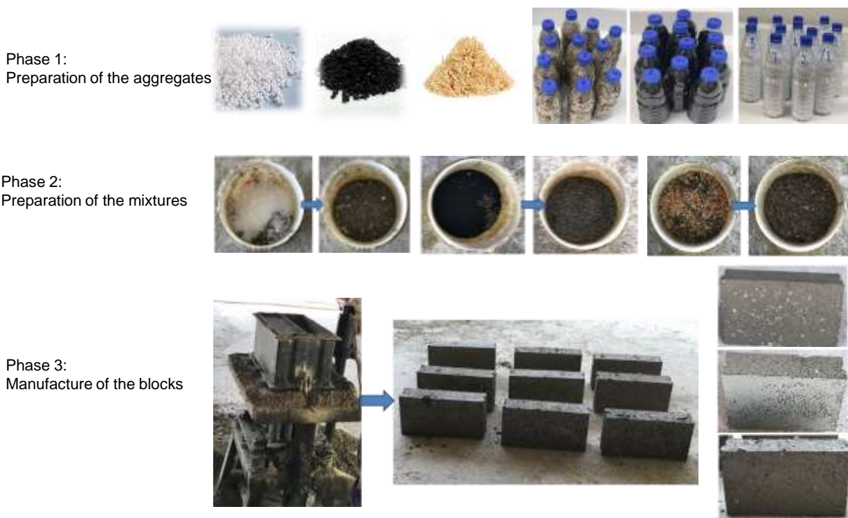
Figure 1- Phases of preparation of the hollow block samples
