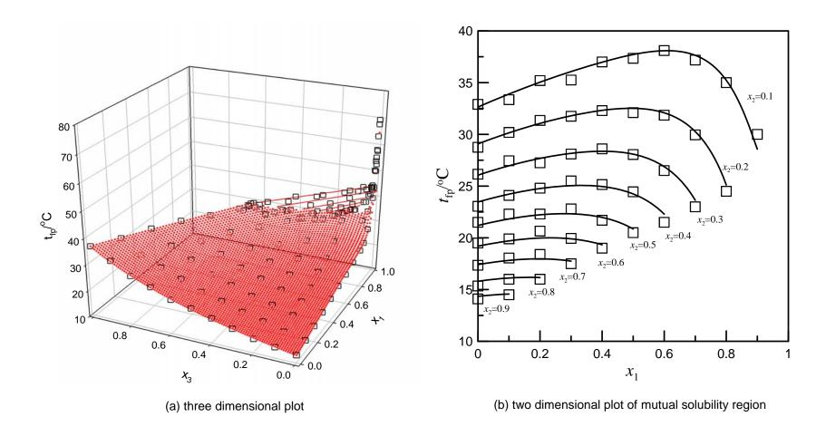
Figure 10. Comparison of predicted flash point and experimental data for water (1) + ethanol (2) + 1-butanol (3).  $\Box$  , experimental data; red  $\cdot$  , mutual solubility region; red  $\overline{\phantom{a}}$  , tie lines.
