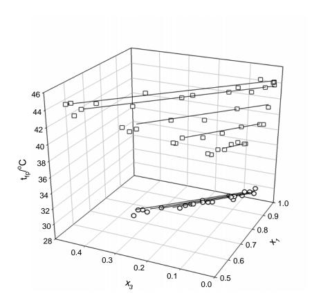
Figure 8. Comparison of predicted flash points in the tie lines with experimental data for water + ethanol + 1-butanol/2-butanol.  $\Box$ , water (1) + ethanol (2) + 1-butanol (3);  $\bigcirc$ , water (1) + ethanol (2) + 2-butanol (3);  $\bigcirc$ , NRTL.
