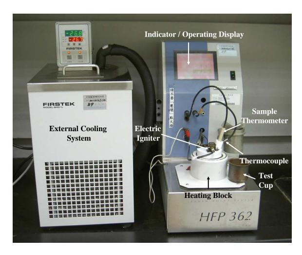
Figure 1. The basic system configuration of the Tag close cup tester.
