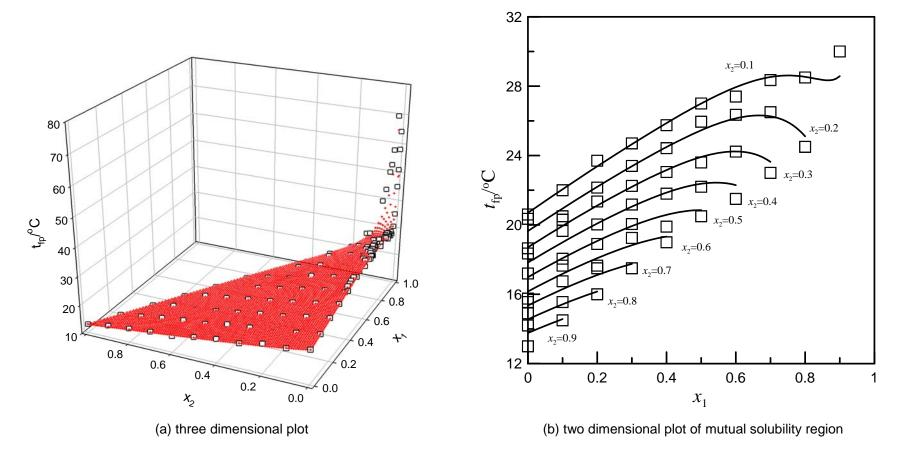
Figure 11. Comparison of predicted flash point and experimental data for water (1) + ethanol (2) + 2-butanol (3).
