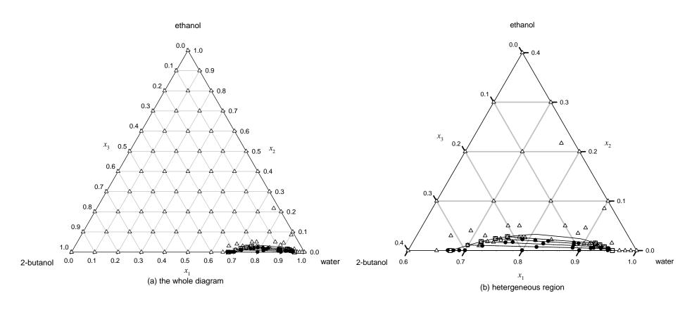
Figure 6. Binodal curves of water (1) + ethanol (2) + 2-butanol (3).  $\bullet$  , partially miscible;  $\triangle$  , miscible;  $\triangle$  , tie line.
