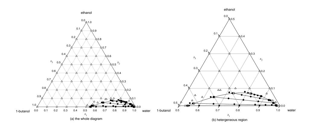
Figure 5. Binodal curves of water (1) + ethanol (2) + 1-butanol (3).  $\bullet$  , partially miscible;  $\triangle$  , miscible;  $\triangle$  , tie line.
