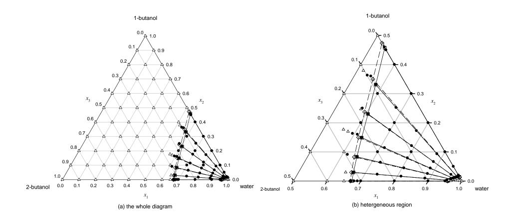
Figure 7. Binodal curves of water (1) + 1-butanol (2) + 2-butanol (3).  $\bullet$ , partially miscible;  $\triangle$ , miscible;  $\triangle$ , miscible;  $\triangle$ , NRTL;  $\diamondsuit$ --- $\diamondsuit$ , UNIQUAC.
