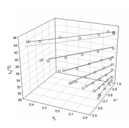
Figure 9. Comparison of predicted flash points in the tie lines with experimental data for water (1) + 1-butanol (2) + 2-butanol (3).  $\Box$ , experimental data;  $\Box$ , NRTL;  $\Box$ , UNIQUAC.
