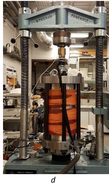
902 Figure 3. a) Enhanced drainage system (with two geotextiles wrapped at top and specimen bottom and put in contact 903 with porous disks) and connections with PVCs; b) Specimen wrapped into top and bottom geotextiles (see Belmokhtar 904 et al. 2018 for more details); c) Autonomous self-compensated HP triaxial cell; d) Timo cell on a 25 tons triaxial press. 905 Both cells are wrapped into an electric red ribbon aimed at controlling temperature at 25°C. 906
