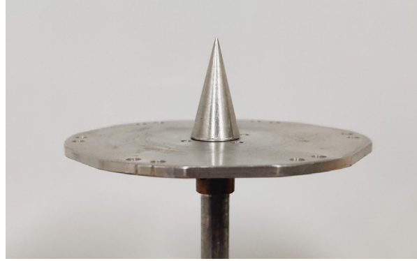
Figure 4. The shape of the SEIS foot. The conical spike has a maximum diameter of 10 mm.
