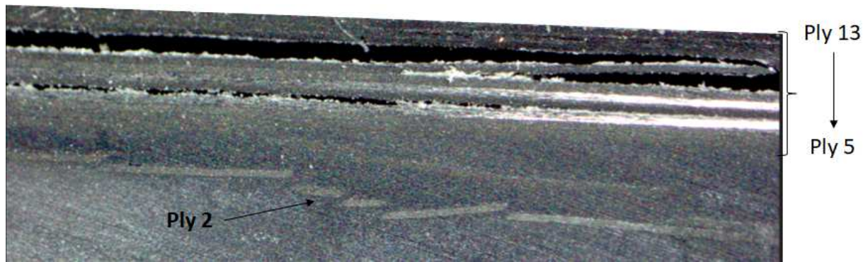
193 Figure 9 Internal damage study for severe configuration: CFRP (13plies) + ECF195 + 1000 \mu m of paint
