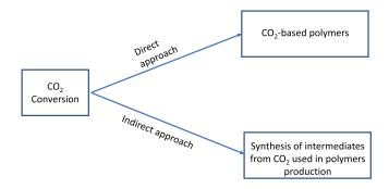
Fig. 2. Approaches for  $CO_2$  conversion into chemicals/polymers.
