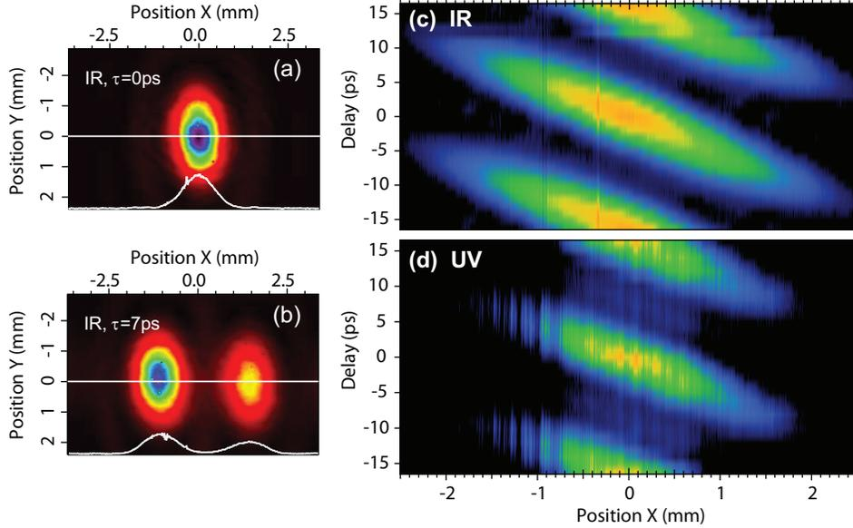
Fig. 8. IR transverse beam profile at the output of the pulse shaper with no modulation (a) and with a linear phase inducing a delay  $\tau = 7$  ps (b). 1D beam profile, i.e. horizontal cut at  $y = 0$ , is depicted in white line on the bottom of each figure. IR (c) and UV (d) 1D beam profile recorded for various applied delays and compiled in a single picture (see text).
