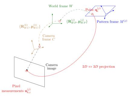
Figure 2. Geometrical representation of the projection camera model.
