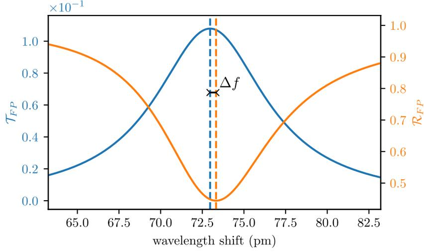
Fig. 1. Calculated reflection and transmission curves of an absorptive Fabry-Perot cavity for two 35 nm thick layers of silver deposited on quartz, with a refractive index  $\tilde{n} = 0.2997283 - i10.7355059$  taken from <https://www.overleaf.com/project/617aa0824dabff9f3a123407> [23]. The resonance is centered close to 1550 nm. The shift in frequency is noticeable here,  $\Delta\lambda = 0,35$  pm which corresponds approximately to  $\Delta f = 45$  MHz.
