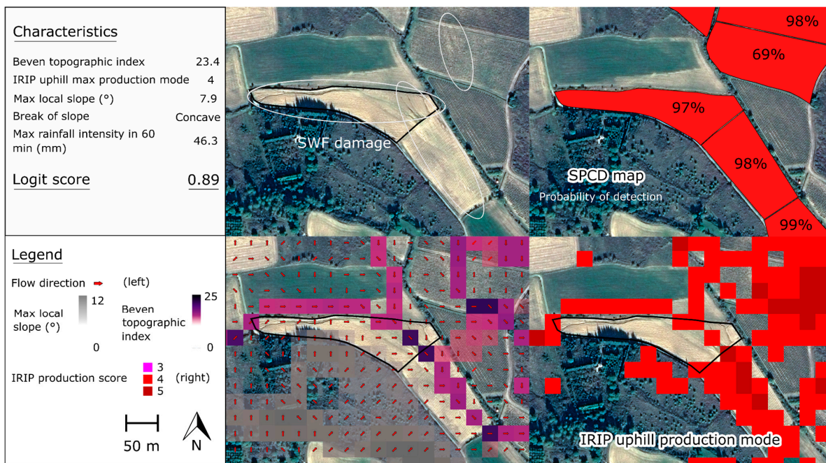
Figure 11. Examples of lands affected by SWF with gullies in Aude. Maximum rainfall intensity in 60 min (Panthere data), associated characteristics used by IRIP and resulting logit score on an affected plot (black contour) can be seen in the top left panel. Top left figure: Pléiades image from 3 November 2018. Top right figure: Probability of damage detection by SPCD method. Bottom left figure: Flow direction, local slope (°) and Beven topographic index (DEM-derived). Bottom right figure: IRIP uphill production mode used in the generation of IRIP accumulation map.
