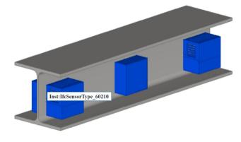
Fig. 15 IfcBeam equipped with three instances of IfcSensor
