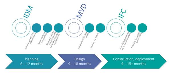
Fig. 1 The building bricks of BIM: IDM, MVD and IFC [3]
