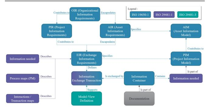
Fig. 14 Standard concepts from ISO 19650-1, ISO 29481-1 and ISO 29481-3 considered by the ANR McBIM ontology
