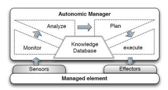
Fig. 10 Illustration of the interactions between an autonomous element and the knowledge base
