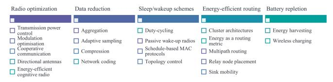
Fig. 3 Approaches addressing energy efficiency in WSNs (adapted from [21])
