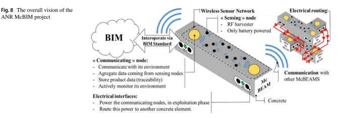
in the ISO 19650 standard family [3, 4, 38-40]. More specifically, the ANR McBIM project aims to design a "communicating concrete", meaning embed concrete building elements with sensors and integrate the sensed data into the BIM platform, thus delivering an interoperable digital building twin (see Fig. 8).
