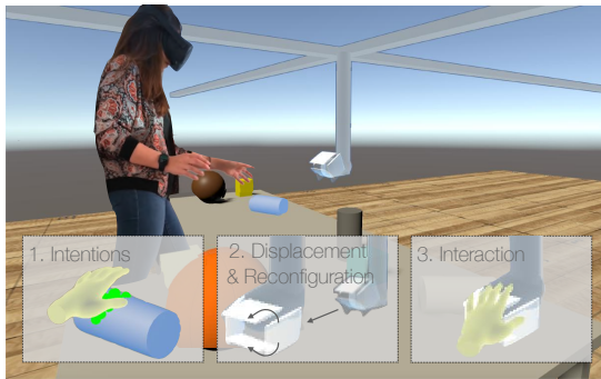
Figure 2: An Encountered-Type of Haptic Device scenario: 1. Intentions, 2. Displacement & Reconfiguration, 3. Interaction.
