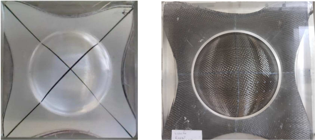
Fig. 13. Hemispherical forming of plain weave and satin weave textile reinforcements.
