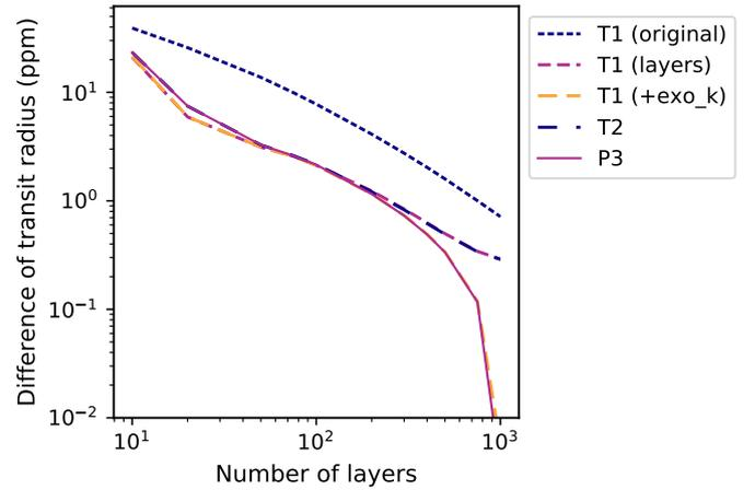
**Fig. 5.** Average of the absolute difference (in ppm) between each model and the converged solution of Pytmosph3R (with 1000 layers) as a function of the number of layers. P3 stands for Pytmosph3R, and T1 and T2 for TauREx 1D and 2D, respectively. The original implementation of TauREx (denoted “T1 (original)”, with rays that are tangent to levels) is included.
