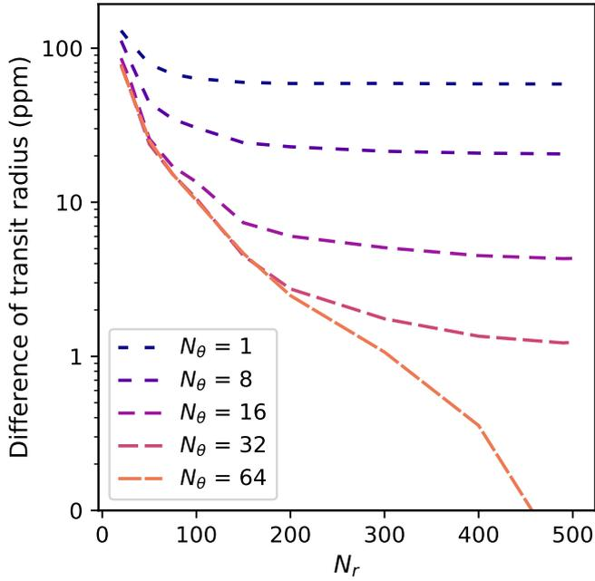
**Fig. 10.** Convergence of Pytmosph3R when the number of rays  $[N_r \times N_\theta]$  crossing the atmosphere is increased, using as a reference point the converged model  $[N_r \times N_\theta] = [500 \times 64]$ . The simulation is a GCM with an equilibrium temperature  $T_{\text{eq}} = 2100$  K based on the characteristics of WASP-121b, and including TiO and VO. The number of cells in this simulation is  $(N_{z,\text{lay}}, N_{\text{lat}}, N_{\text{lon}}) = (100, 32, 64)$ .
