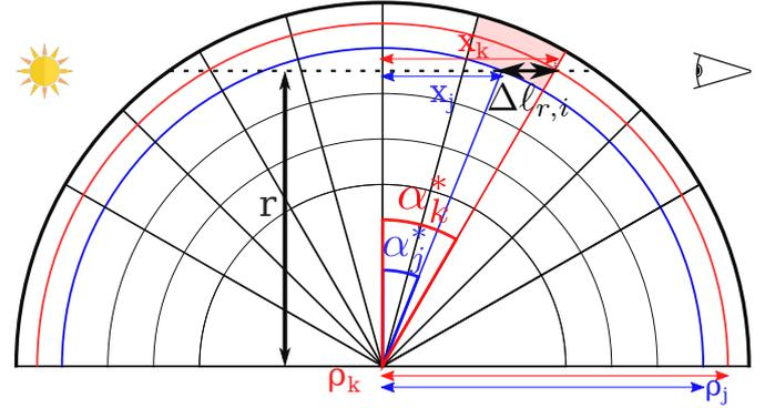
**Fig. 3.** Intersection of a ray with the 2D grid. An example of intersections for one level and one angle is highlighted by points  $j$  and  $k$  at coordinates  $(\rho_j, \alpha_j^*)$  and  $(\rho_k, \alpha_k^*)$ , respectively. The length  $\Delta\ell_{r,i}$  of the corresponding segment is deduced from the computation of the distances  $x_j$  and  $x_k$  of both points to the terminator. The coordinates of the segment must also be computed to obtain the physical properties of the cell.
